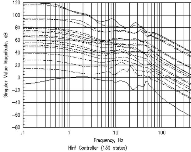
The 130 state HAC<sub>∞</sub> compensator was reduced to a 60 state HAC<sub>∞</sub> compensator by applying frequency-weighted balanced truncation to the error measure
